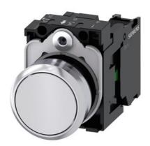
Pushbutton, 22 mm, round, metal, shiny, white, pushbutton, flat, momentary contact type, 1 NO, screw terminal, with laser labeling, upper case and lower case, always upper case at beginning of line
