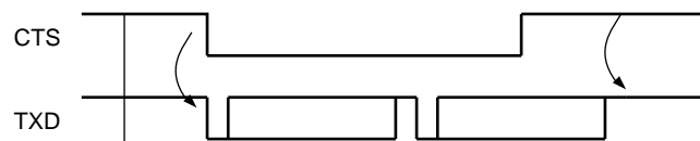
Figure 36-28. Transmitter Behavior when Operating with Hardware Handshaking
