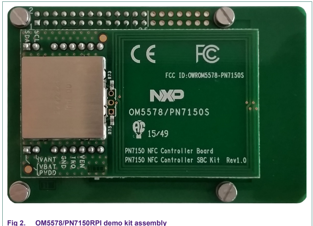
Fig 2. OM5578/PN7150RPI demo kit assembly
