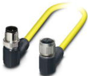
Sensor/actuator cable, 5-position, PVC, yellow, shielded, Plug angled M12 SPEEDCON, A-coded, on Socket angled M12 SPEEDCON, A-coded, cable length: 1.5 m
