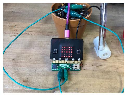
This example uses the Bonsai Buckaroo, the micro:bit, and Microsoft MakeCode to create an automatic plant care system.
