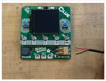
Wire the Pump Driver Terminal The Bonsai Buckaroo terminal connectors are springloaded press-fit connectors. Push down on one tab to separate the internal connector a bit and then push in the wire. Release the pressure on the tab and the terminal will grip the wire.
