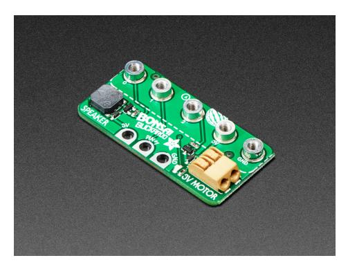
We can't wait for spring to arrive, and we're looking forward to caring for some plants! We designed this little add-on for micro:bit (https://adafru.it/JFI)or CLUE (https://adafru.it/JFJ) boards – bolt it on with 5 screws to get a buzzer/beeper, motor driver, and breakouts for connecting a soil sensor (https://adafru.it/JFK) (two alligator clips + nails work just fine). Simple, but effective!
