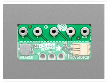
Along the top are the **mount points**. The Bonsai Buckaroo ships with screws for attaching to your micro:bit or CLUE.
