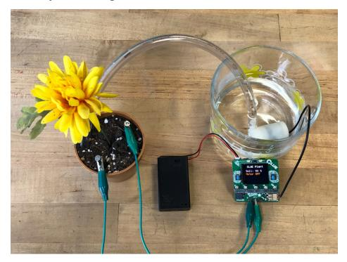
It's easy to use the Adafruit Bonsai Buckaroo with CircuitPython. This example uses the Adafruit CircuitPython CLUE (https://adafru.it/JFL) library to display soil moisture level and the status of the pump motor on the CLUE display. Connect your Bonsai Buckaroo to your CLUE, and connect the motor and plant to the Bonsai Buckaroo, and you're on your way to automatic plant care. Let's take a look!
