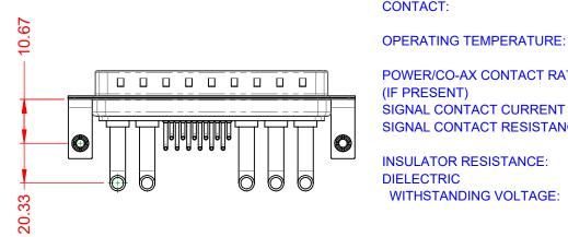
40A (CURRENT) POWER/CO-AX CONTACT RATING: (IF PRESENT) SIGNAL CONTACT CURRENT RATING: 5A PER CONTACT SIGNAL CONTACT RESISTANCE:  $10m\Omega$  MAX. **INSULATOR RESISTANCE:** 5000MΩ min.
