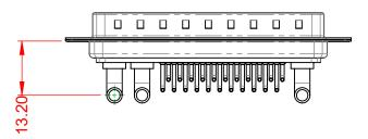
POWER/CO-AX CONTACT RATING: 40A (CURRENT) (IF PRESENT) SIGNAL CONTACT CURRENT RATING: 5A PER CONTACT SIGNAL CONTACT RESISTANCE:  $10m\Omega$  MAX. INSULATOR RESISTANCE:  $5000M\Omega$  min. DIELECTRIC
