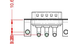
**OPERATING TEMPERATURE:** -55°C ~ 125°C 30A (CURRENT) POWER/CO-AX CONTACT RATING: (IF PRESENT) SIGNAL CONTACT CURRENT RATING: 5A PER CONTACT SIGNAL CONTACT RESISTANCE:  $10m\Omega$  MAX. **INSULATOR RESISTANCE:** 5000MΩ min.
