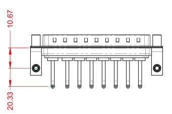
**OPERATING TEMPERATURE:** -55°C ~ 125°C 10A (CURRENT) POWER/CO-AX CONTACT RATING: (IF PRESENT) SIGNAL CONTACT CURRENT RATING: 5A PER CONTACT SIGNAL CONTACT RESISTANCE:  $10m\Omega$  MAX. **INSULATOR RESISTANCE:** 5000MΩ min. DIELECTRIC
