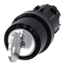
RONIS key-operated switch, 22 mm, round, plastic, lock number 455, with 2 keys, 3 switch positions I-O-II, latching, actuating angle 2x45°, 10:30h/12h/13:30h, Key removal I+O+II, with laser labeling, inscription or symbol Customer-specific selection with SIRIUS ACT configurator (CIN)
