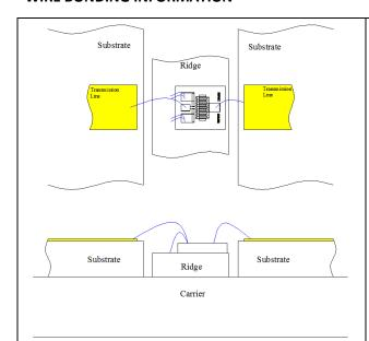
Using 1 mil. diameter, Au bonding wires.
