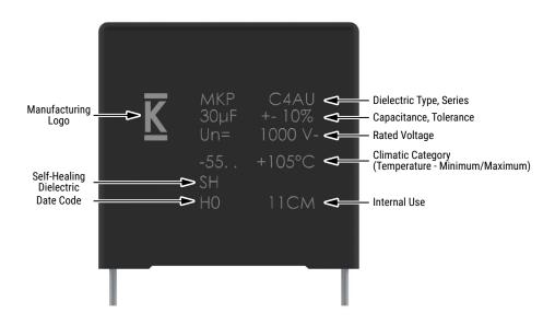
Slight change in the layout can be possible but this does not affect the content of the information of the current marking.
