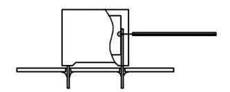
Temperature monitored inside the capacitor.
