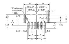
(Tolerance: ±0.05) Note: The overall pattern pitch tolerance for the board is  $\pm 0.05$ . Do not accumulate error. \* The 1-mm diameter holes are for the positioning bosses. Use metal masks to prevent solder from entering these holes.
