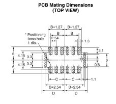
(Tolerance: ±0.05) Note: The overall pattern pitch tolerance for the board is ±0.05. Do not accumulate error The 1-mm diameter holes are for the positioning bosses. Use metal masks to prevent solder from entering these holes.
