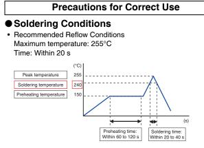
These conditions depend on the type of solder, the manufacturer, the amount of solder, the size of the circuit board, and the other mounting materials. You must check and select the actual conditions yourself.
