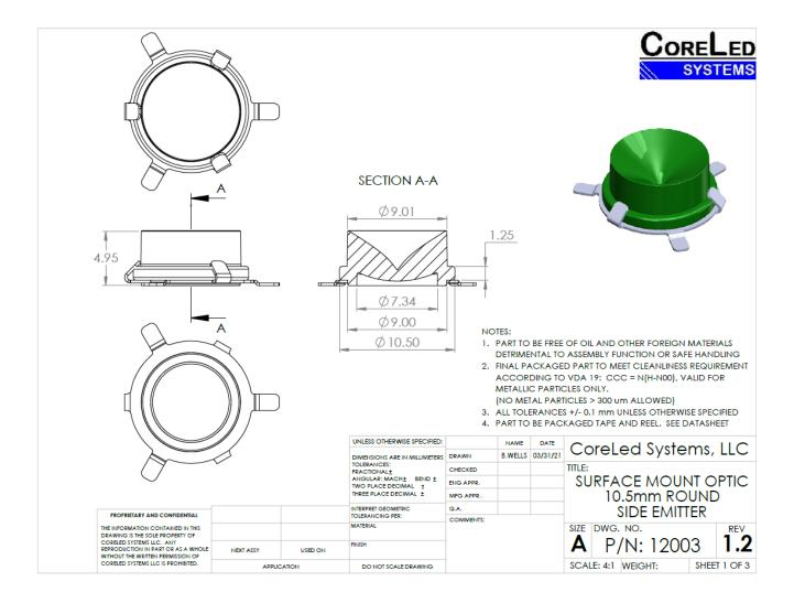
Mechanical design features shown with solder clip
