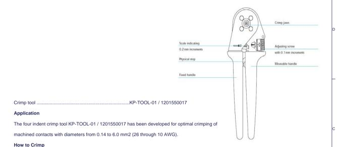
The reference table indicates the correct locator position to be selected and the crimp depth to be adjusted for the contact to be crimped. The contact is then inserted through the access hole of the tool on the opposite side of the locator. The contact is held in place by closing the handles to the first lock-in position thus preventing the contact from falling out of the tool and facilitating insertion of the wire into the contact.
