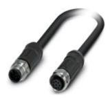
Sensor/actuator cable, 8-position, PE-X/PE-X halogen-free, black-gray RAL 7021, shielded, Plug straight M12, A-coded, on Socket straight M12, A-coded, cable length: 2 m, for outdoor applications, with high-grade steel knud
