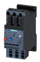
Overload relay 27...32 A Thermal For motor protection Size S0, Class 10 Stand-alone installation Main circuit: Spring-type terminal Auxiliary circuit: spring-type terminal Manual-Automatic-Reset
