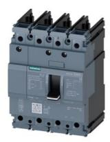
circuit breaker 3VA5 UL frame 125 breaking capacity class S 25kA @ 480V 4-pole, line protection TM210, FTFM, In=90A overload protection Ir=90A fixed short-circuit protection Ii=10 x In N conductor protection 100% without connection
