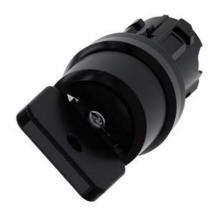
Key-operated switch O.M.R, 22 mm, round, plastic, lock number 73034, black, with 2 keys, 2 switch positions O<I, momentary contact type, Actuating angle 45°, 10:30h/12h, key removal O, with laser labeling, upper case and lower case, always upper case at beginning of line
