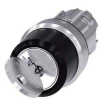
RONIS key-operated switch, 22 mm, round, metal, shiny, lock number SB30, with 2 keys, 2 switch positions O-I, latching, actuating angle 90°, 10:30h/13:30h, key removal O+I, possible special locks: SB31, 421, 455, with laser labeling, upper case and lower case, always upper case at the beginning of the word
