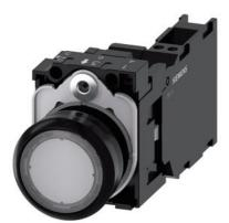
Illuminated pushbutton, 22 mm, round, plastic, clear, pushbutton, flat, momentary contact type, with holder, 1 NO+1 NC, LED module with integrated LED 24 V AC/DC, spring-type terminal, with laser labeling, symbol number according to, ISO 7000 or IEC 60417
