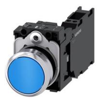
Pushbutton, 22 mm, round, metal, shiny, blue, pushbutton, flat, momentary contact type, 1 NO+1 NC, spring-type terminal, with laser labeling, upper case and lower case, always upper case at beginning of line
