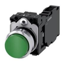
Pushbutton, 22 mm, round, metal, shiny, green, pushbutton, raised, momentary contact type, with holder, 1 NO+1 NC, screw terminal, with laser labeling, symbol number according to, ISO 7000 or IEC 60417
