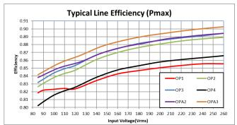
An estimate of the efficiency for any particular system may be obtained from these graphs using the procedure outlined in the example below.
