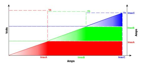
In this mode the highest adjusted output module will supply all of the load current until its current limit is reached. If the
