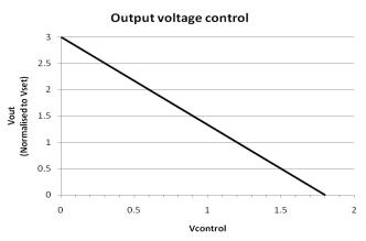
The output voltage can be controlled from 0% to 300% of the preset voltage using this control method. However, care must be taken to ensure the output voltage does not exceed the OVP level, as this is considered a safety hazzard and will latch the entire unit off. To determine the level of control voltage that will trigger OVP, insert Vovp into the equation above.
