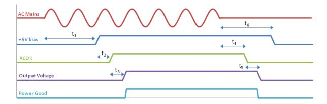
Typical timing values at 25°C:  $t_1\phi$  2000 ms,  $t_2\phi$  50 ms,  $t_3\phi$ 25 ms,  $t_4\phi$  15 ms,  $t_5$  = 5 ms (minimum),  $t_6\phi$  100 ms
