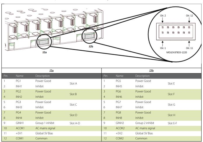
Note that for modules requiring more than 1 slot, the INHx and PGx use the highest number available for x. The other controls will have no function. E.g. For an OPA2 fitted in slots AB, INH1 & PG1 have no function while INH2 and PG2 provide the usual functions for the module.
