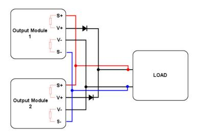
Typically, this configuration can damage the internal sense resistors used within a power supply. However, the NEVO outputs have integrated protection to prevent this type of damage and are completely N+1 compatible without any additional external protection circuitry. Note that only the positive sense terminal is protected and diodes should be used in the positive connection only.
