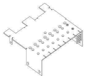
Place the lid back onto the chassis base. Ensure the PCB of each Output Module fits into the corresponding slot on the chassis lid. Secure all the screws.
