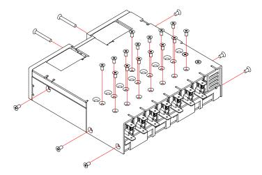
Once all the screws are fully secured attach the power cord and switch on the main supply voltage. Ensure that the Green LED light on each Output Module comes on. As per step 5, measure the output voltage of each output module and adjust to the desired voltage by adjusting the potentiometer below the positive output terminal (top terminal).
