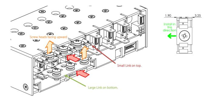
For the NEVO+1200 unit a set of jumper links are also available. By using these jumper links up to eight modules can be connected in parallel. Connect jumper link as shown below and ensure the screws are properly tightened.
