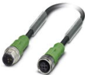
Sensor/actuator cable, 3-position, PUR halogen-free, black-gray RAL 7021, Plug straight M12, A-coded, on Socket straight M12, A-coded, cable length: 5 m, For valve connector
