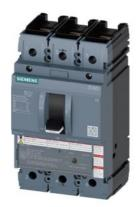
circuit breaker 3VA5 UL frame 250 breaking capacity class H 65kA @ 480 V 3-pole, line protection TM230, FTAM, In=70A overload protection Ir=70A fixed short-circuit protection Ii=5...10 x In UL489 SB (naval), 50 deg. cel. nut keeper kit on both sides
