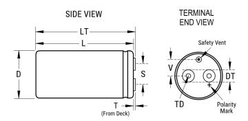
General Information Series ALS70 Dielectric Aluminum Electrolytic Description Screw Terminal, Aluminum Electrolytic RoHS AEC-Q200 No Halogen Free Yes Component 615 g Weight Dimensions D And L Include Sleeving. MS (MxH) = Notes M12x16. Mounting Clamp (Sold Separately): V90N Shelf Life 156 Weeks
