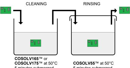
5 minutes submerged 30 second drip dry above 5 minutes submerged 30 second drip dry above
