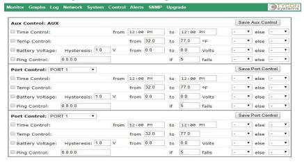
This is where you can setup ping control and other available controls for the ports. The controls are separate into 1 set of controls for the Auxiliary port and another set of controls for the PoE ports. Controls available are Time Control, Temperature Control, Battery Voltage Control, and Ping Control. You can use multiple controls providing for compound functionality. When more than 1 control is enabled, the priority is top to bottom.
