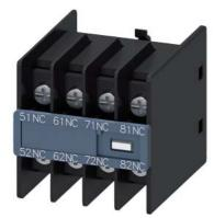
Auxiliary switch on the front, 4 NC Current path 1 NC, 1 NC, 1 NC, 1 NC for contactor relays Size S00 Ring cable lug connection 53/54, 63/64, 73/74, 83/84 Physically coded; only with contactor relays 3RH2140\* and 3RH2440\* can be combined (according to EN 50011)
