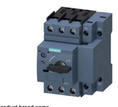
Circuit breaker size S0 for motor protection, CLASS 10 with overload relay function A-release 16...22 A N-release 286 A screw terminal Standard switching capacity
