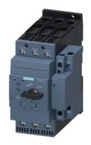
Circuit breaker size S2 for motor protection, CLASS 10 with overload relay function A-release 49...59 A N-release 845 A Standard switching capacity
