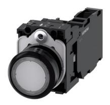
Illuminated pushbutton, 22 mm, round, plastic, clear, pushbutton, flat, momentary contact type, with holder, 1 NO+1 NC, LED module with integrated LED 24 V AC/DC, screw terminal
