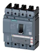
circuit breaker 3VA5 UL frame 250 breaking capacity class C 100kA @ 480V 4-pole, line protection TM210, FTFM, In=200A overload protection Ir=200 A fixed short-circuit protection li=10 x In N conductor protection 100% without connection
