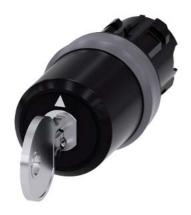
key-operated switch Siemens, 22 mm, round, plastic with metal front ring, lock number SSG10, with 2 keys, 3 switch positions I-O-II, latching, actuating angle  $2x45^{\circ}$ , 10:30h/12h/13:30h, key removal O, Z=50-unit packaging
