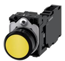
Pushbutton, 22 mm, round, plastic, yellow, pushbutton, flat, momentary contact type, with holder 1 NO+1 NC, screw terminal, with laser labeling, upper case and lower case, always upper case at the beginning of the word
