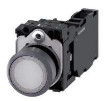
Illuminated pushbutton, 22 mm, round, plastic with metal front ring, white, pushbutton, flat, momentary contact type, with holder, 1 NO+1 NC, LED module with integrated LED 24 V AC/DC, screw terminal, with laser labeling, symbol number according to, ISO 7000 or IEC 60417
