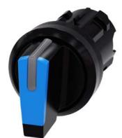
Selector switch, illuminable, 22 mm, round, plastic, blue, selector switch, short, 3 switch positions I-O<II, left latching, right momentary contact type, actuating angle  $2x45^{\circ}$ , 10:30h/12h/13:30h Z=50-unit packaging
