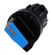
Selector switch, illuminable, 22 mm, round, plastic, blue, selector switch, short, 2 switch positions O-I, latching, actuating angle 90°, 10:30h/13:30h, with laser labeling, upper case and lower case, always upper case at the beginning of the word
