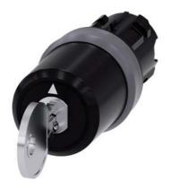
key-operated switch Siemens, 22 mm, round, plastic with metal front ring, lock number SSG10, with 2 keys, 3 switch positions I-O-II, latching, actuating angle 2x45°, 10:30h/12h/13:30h, key removal O+I, Z=50-unit packaging
