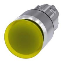
Illuminated mushroom pushbutton, 22 mm, round, metal, shiny, yellow, 30 mm, latching, pull-to-unlatch mechanism, Z=50-unit packaging
