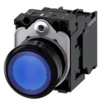
Illuminated pushbutton, 22 mm, round, plastic, blue, pushbutton, flat, momentary contact type, with holder, 1NO, LED module with integrated LED 110 V AC, screw terminal, Z=20-unit packaging
