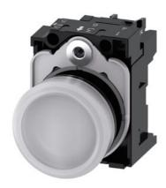
Indicator lights, 22 mm, round, plastic, white, lens, smooth, with holder, LED module with integrated LED 110 V AC, screw terminal, Z=20-unit packaging
