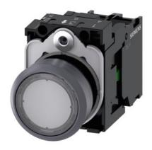
Illuminated pushbutton, 22 mm, round, plastic with metal front ring, clear, pushbutton, flat, momentary contact type, with holder, 1NO, LED module with integrated LED 110 V AC, screw terminal, with laser labeling, upper case
