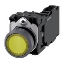
Illuminated pushbutton, 22 mm, round, plastic with metal front ring, yellow, pushbutton, flat, momentary contact type, with holder, 1 NO+1 NC, LED module with integrated LED 110 V AC, screw terminal, with laser labeling, lower case
