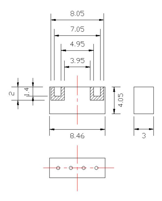
Dimensions in mm Tolerance:±0.25
