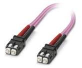
Assembled FO cable, zip cord cable, multi-mode fiberglass 50/125  $\mu$ m, OM4, plug: SC-RJ/SC-RJ, degree of protection: IP20, for installation in cable ducts or control cabinets, length: 2 m
