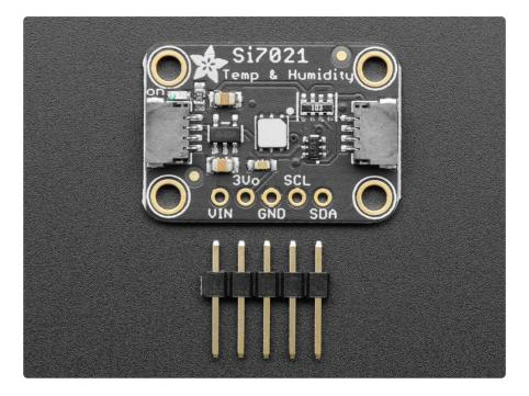
There's a PTFE filter to keep the sensor clean, that's the white flat thing on top. Also comes with some pin header. Some light soldering is required to attach the header for use in a breadboard but it's easy to do.
