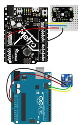
Connect Vin to the power supply, 3-5V is fine. (red wire on STEMMA QT version) Use the same voltage that the microcontroller logic is based off of. For most Arduinos, that is 5V Connect GND to common power/data ground (black wire on STEMMA QT version)
