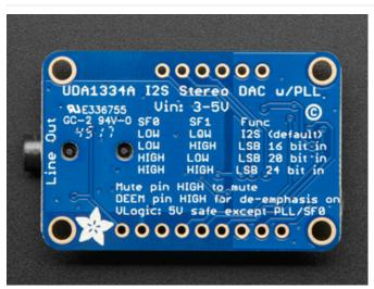
**SF0** and **SF1** are used to set the input data format. By default both are pulled Low for I2S but you can change them around for alternate formats.
