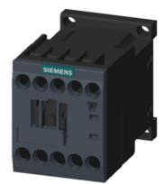
Power contactor, AC-3 16 A, 7.5 kW / 400 V 1 NC, 380 V AC, 50/60 Hz 3-pole, Size S00 screw terminals
